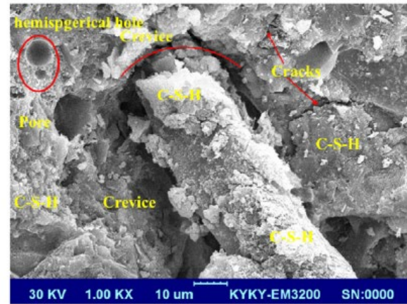
(b) CTF reinforced concrete
