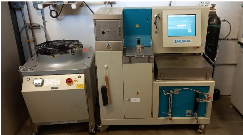
Figure 2.11: Closed loop binder extraction system.
