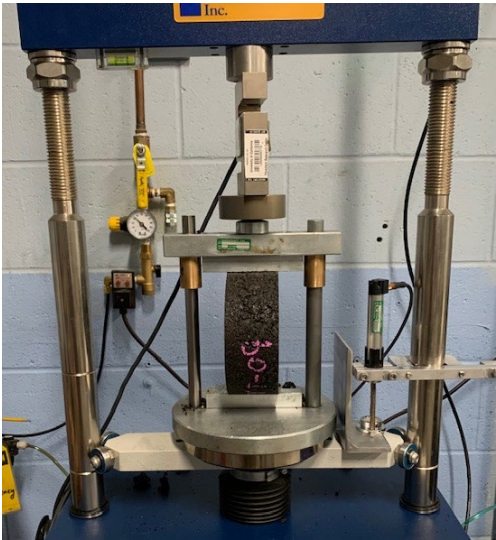
Figure 2.15: Testing machine for IDEAL-CT with a specimen.
