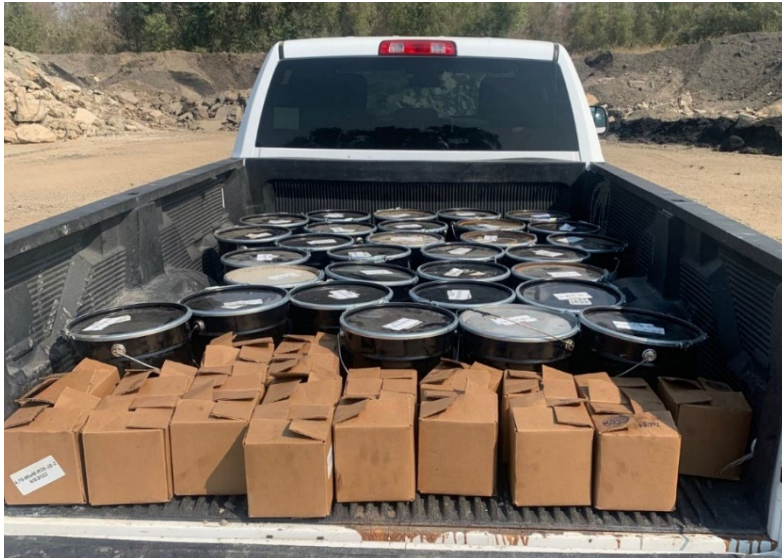
Figure 2.9: Samples from job mix formula submittal of one mix loaded into the back of a truck.
