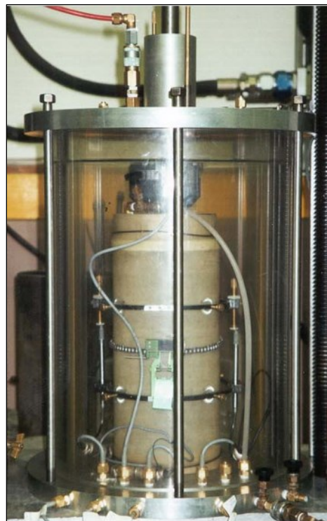
Figure 2.9: Triaxial test setup with on-specimen LVDTs and a radial extensometer.
