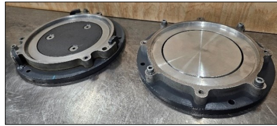
Figure 4.5: Original and new base plate for Wirtgen cell (new plate on left).
