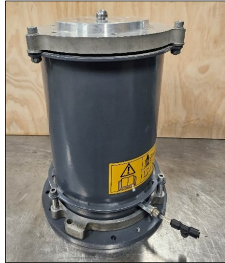
Figure 4.3: Assembled Wirtgen confinement cell with the new loading platen.
