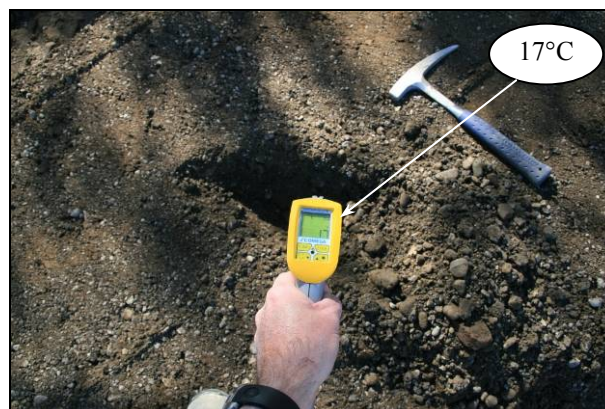
Figure 7.27: Recycled material (cold).
