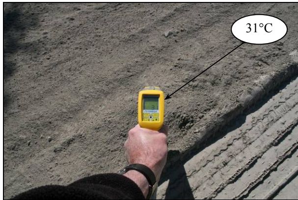
Figure 7.28: Cement temperature prior to recycling (warm).
