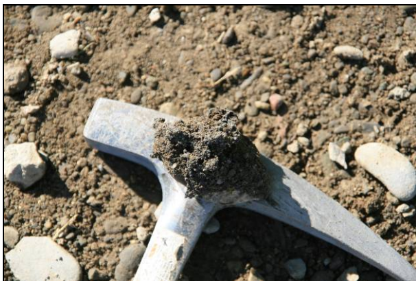
Figure 7.30: Poor asphalt dispersion on cold aggregate.
