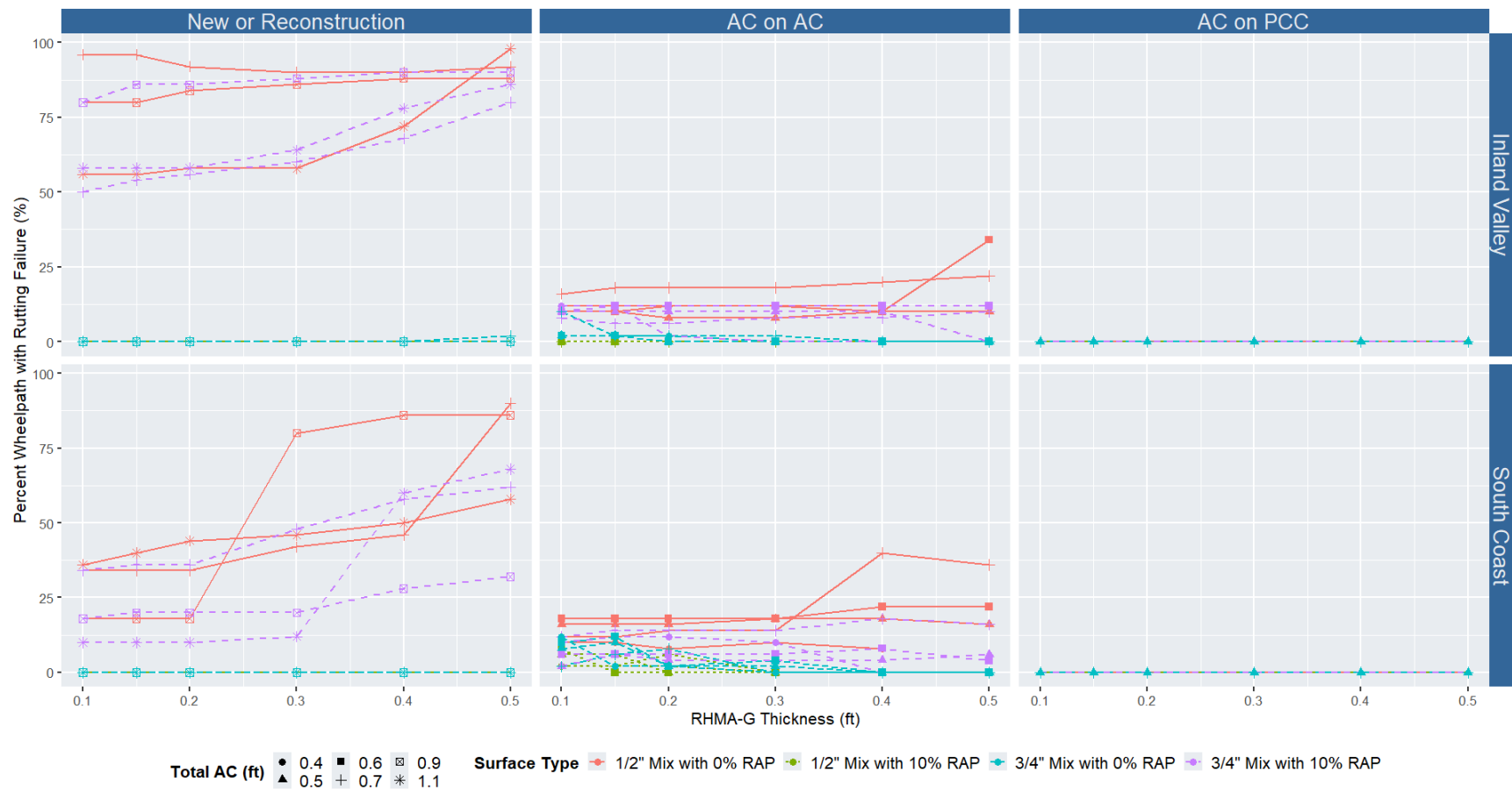
Figure D.13: Percent wheelpath with rutting failure at the end of pavement life.
