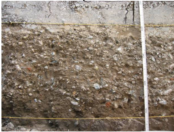
Figure 3.48: 588RF#12 weaker cemented base material.
