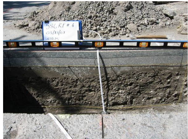
Figure 3.29: 586RF#4 test pit profile.
