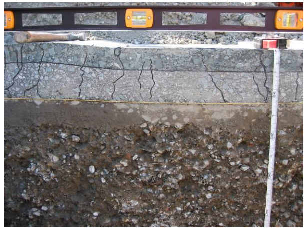
Figure 3.35: 587RF#4 test pit profile.
