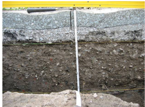
Figure 3.25: 584RF test pit profile. (3)
