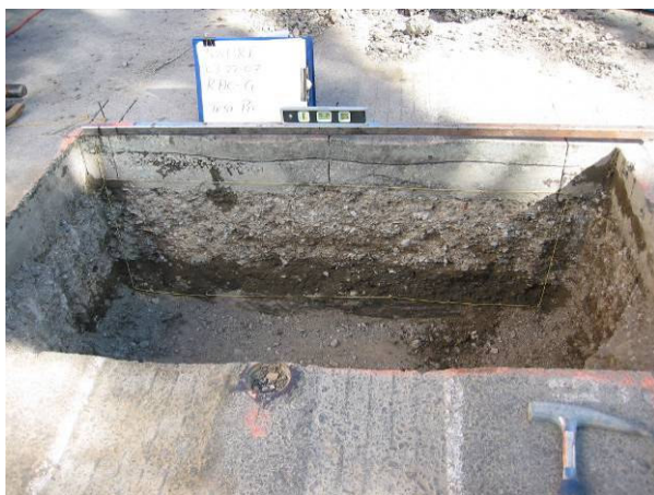
Figure 3.12: 581RF test pit profile. (2)
