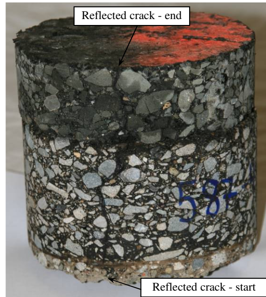
Figure 3.71: RAC-G: Cracks on core.
