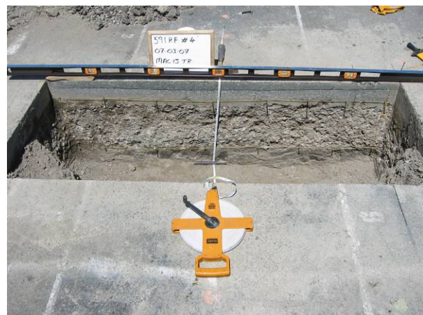
Figure 3.63: 591RF#4 test pit profile.
