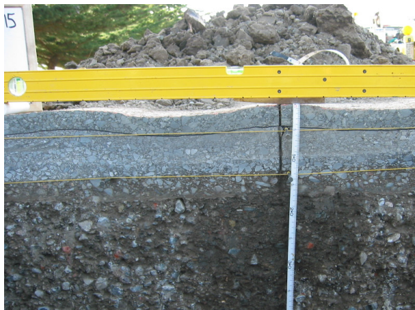
Figure 3.5: 580RF test pit profile. (3)
