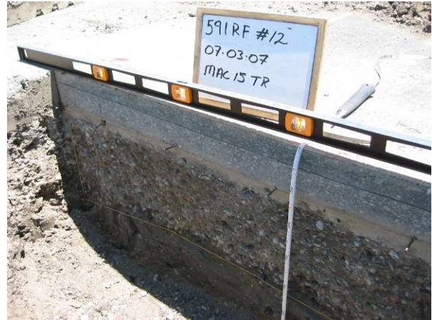
Figure 3.65: 591RF test pit profile.
