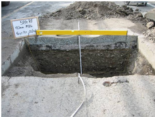
Figure 3.24: 584RF test pit profile. (2)
