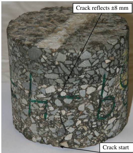
Figure 3.74: 45 mm MB4-G: Cracks on core.
