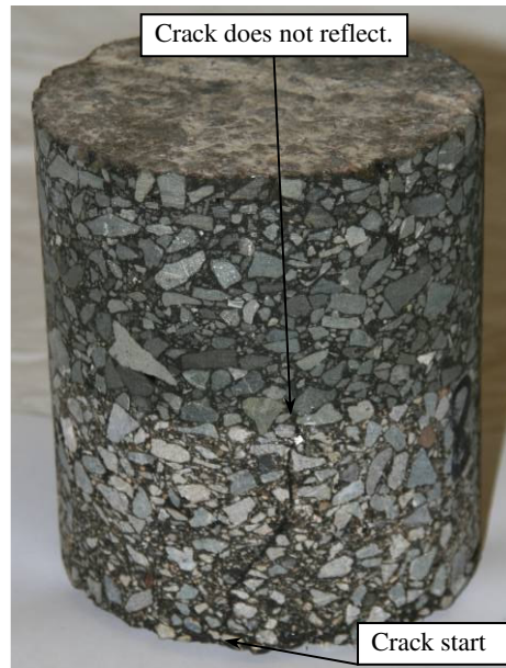
Figure 3.75: 90 mm MB4-G: Cracks on core..
