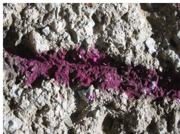
Figure 3.7: 580RF phenolphthalein reaction.
