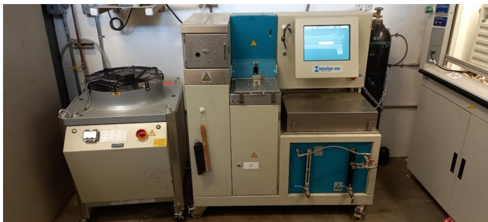
Figure 2.7: Closed-loop binder extraction system.
