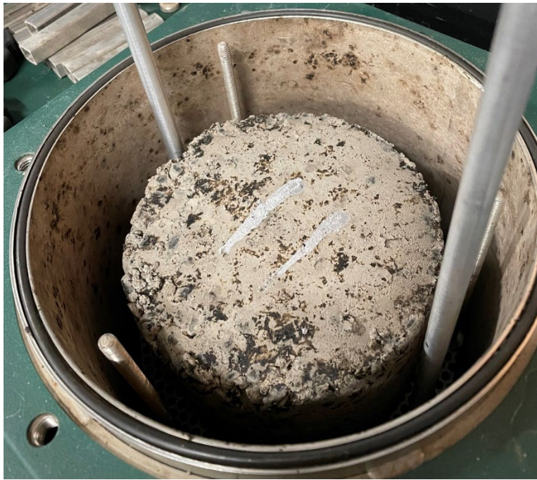
Figure 2.19: Specimens in the MiST 2 device.
