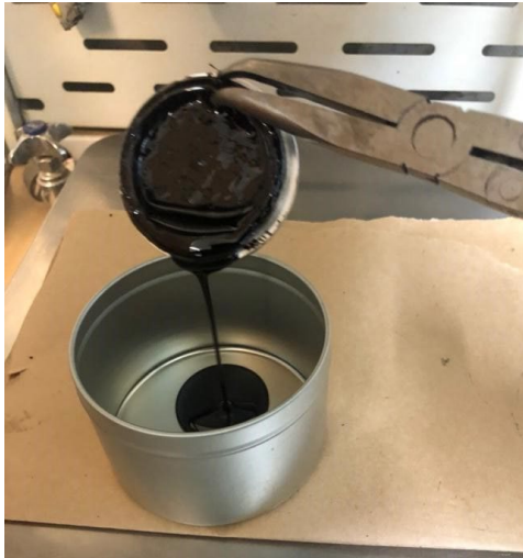
Figure 2.12: Removing the binder from the cup after centrifuging out the rubber particles.
