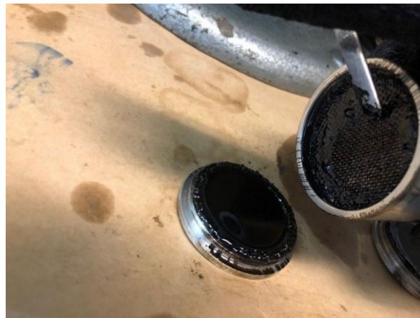
Figure 2.13: Removing the residual rubber particles from the centrifuge cup.
