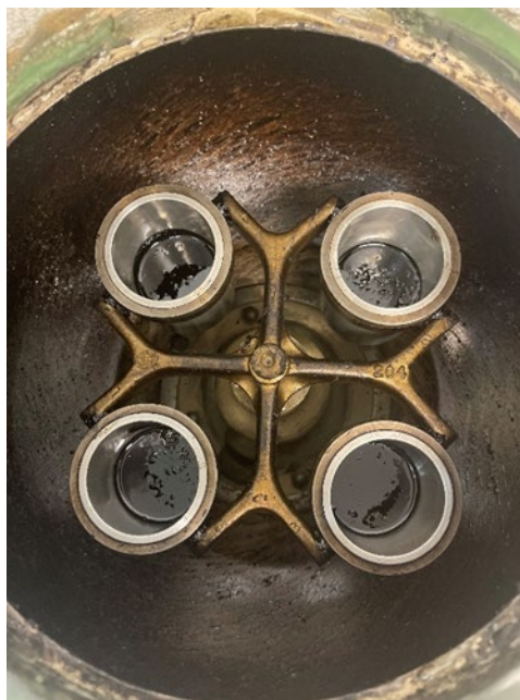
Figure 2.11: Cups with binder in centrifuge prior to centrifuging.
