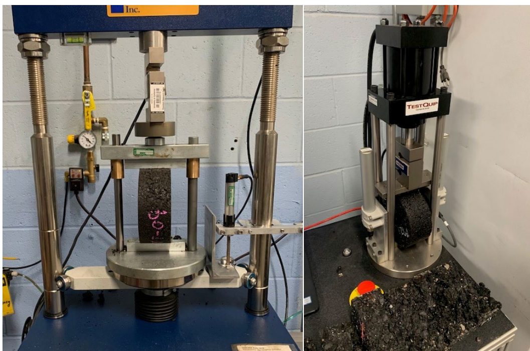
Figure 2.15: Testing machine for IDEAL-CT test with a specimen.
