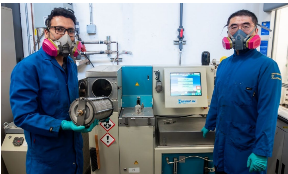
Figure 2.8: Placing extraction cylinder with sample into extraction system.
