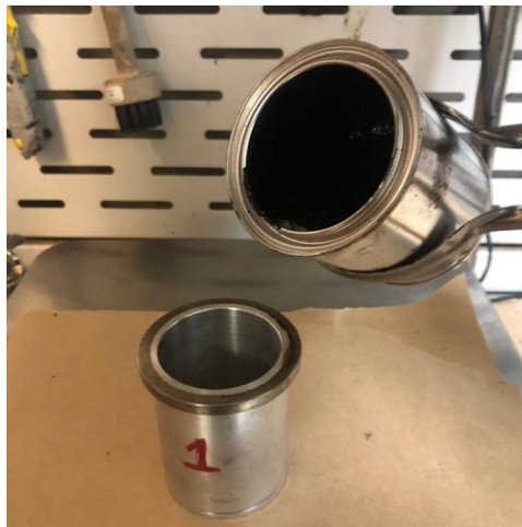
Figure 2.10: Pouring heated rubberized asphalt into centrifuge cup.
