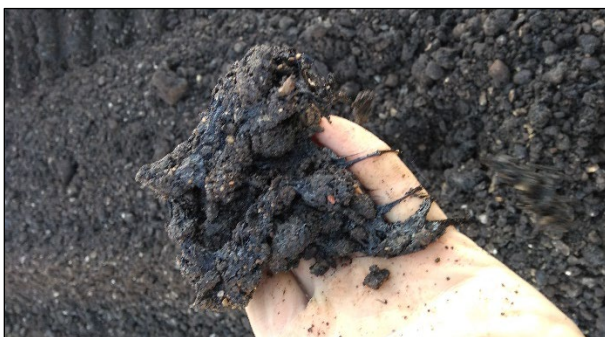
Figure 6.44: Poorly dispersed asphalt recycling agent (nozzle problem).
