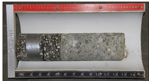
Figure 2.44: Asphalt on cement-treated base.
