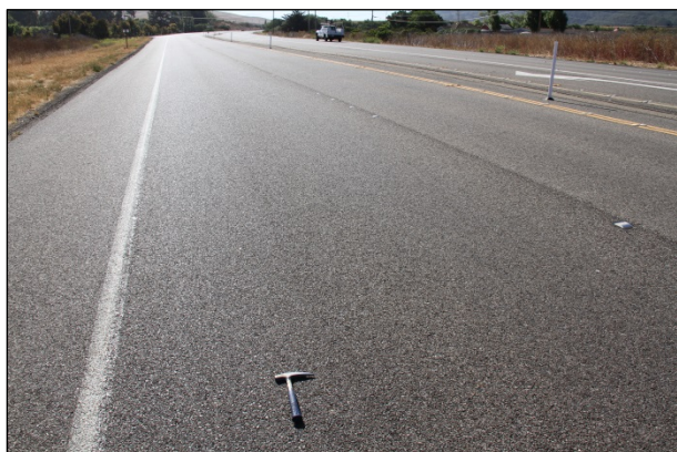
Figure 3.10: Morro Bay Evotherm, May 2012 (60 months), track marks no longer visible.
