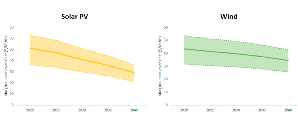
Figure 5. Implied marginal breakeven costs (2018 US$/MWh) for solar PV and wind relative to new coal generation, LDHR scenario
