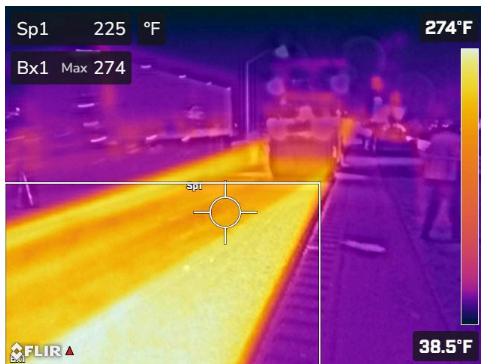
Figure 5.11: Second image of mat after breakdown.
