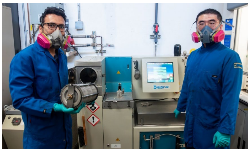
Figure 2.14: Placing extraction cylinder with sample into extraction system.
