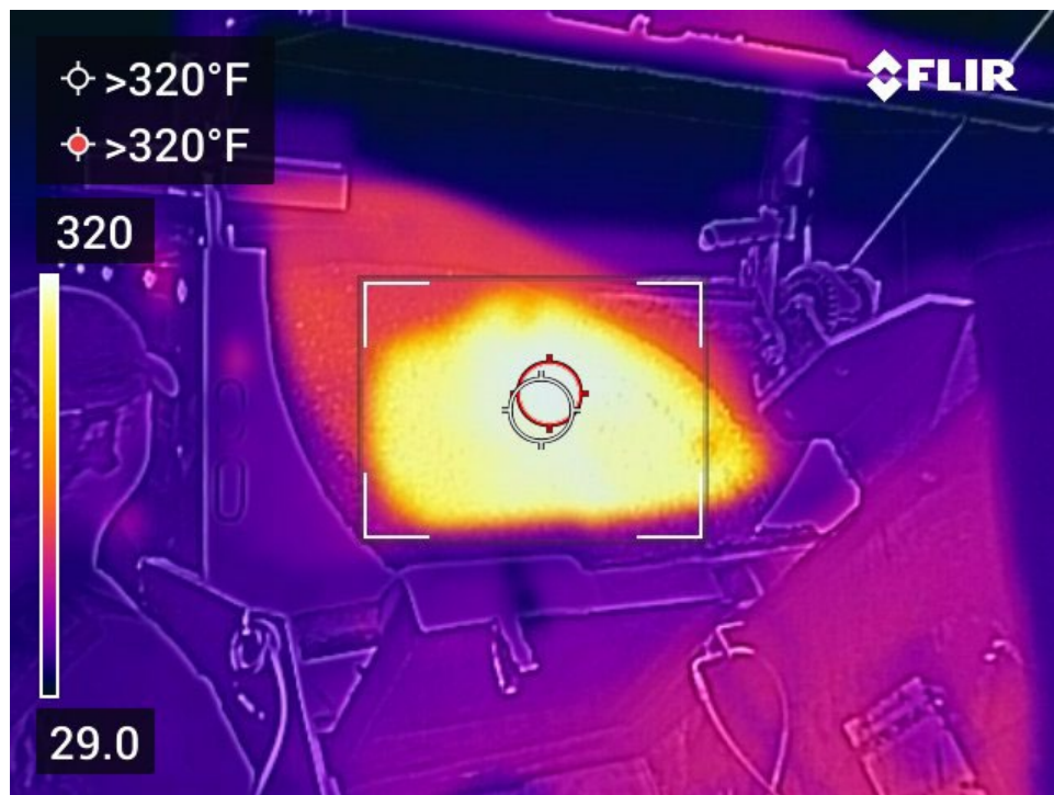
Figure 5.6: Thermal image of placement of mix into shuttle buggy.
