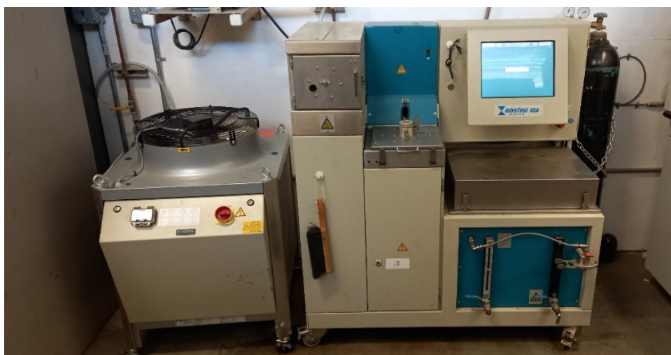
Figure 2.13: Closed-loop binder extraction system.
