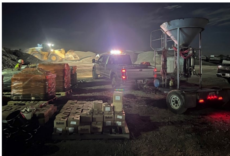
Figure 2.12: Loose plant mix samples stored in cardboard boxes on SBD 215.
