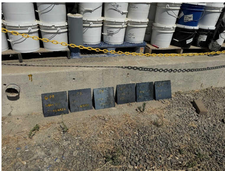
Figure 3.32: GPR metal tracing plates.
