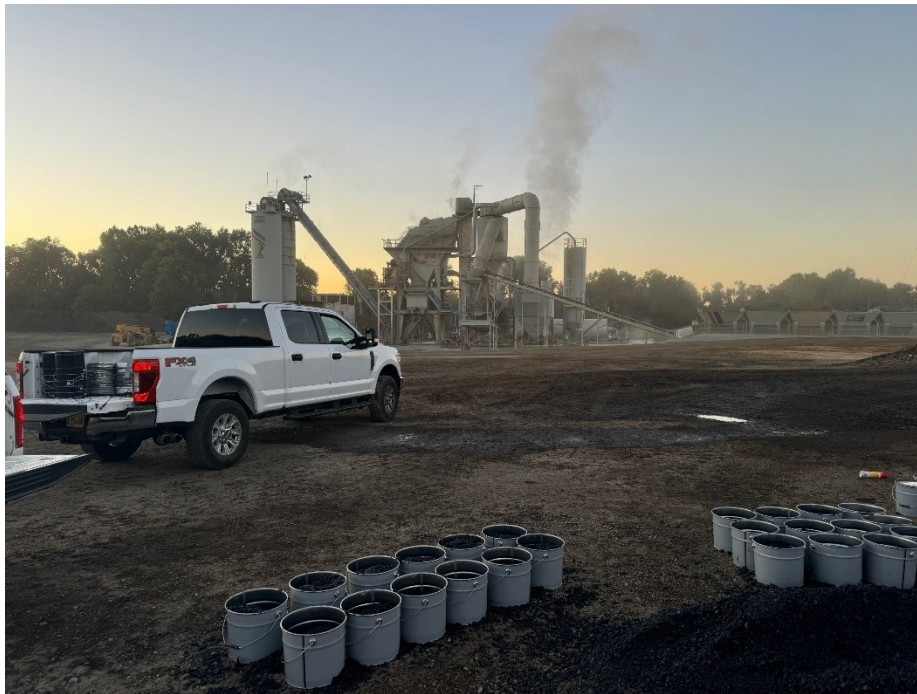
Figure 4.1: Hot drop sampling at George Reed Inc. batch plant in Clements.
