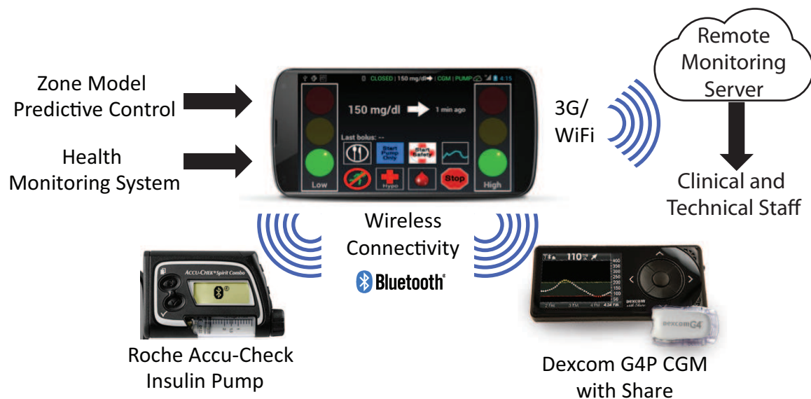
Figure 2.1: Components of the ZMPC+HMS/DiAs system. The ZMPC+HMS algorithms are hosted on the DiAs platform, which runs on medical Android on a Nexus 5 phone. The DiAs platform communicates with the Roche Accu-Chek insulin pump and the Dexcom G4P CGM via Bluetooth. The DiAs platform also communicates with the DiAs Web Monitoring site by 3G or internet connection.
