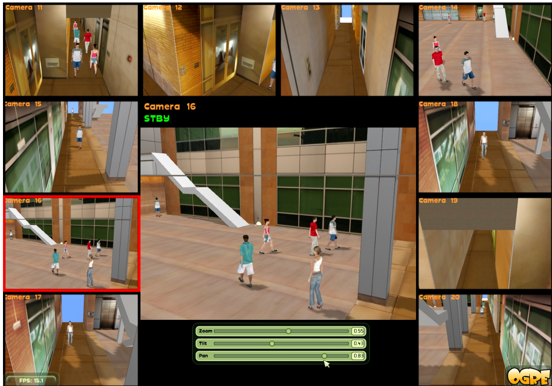
Figure D.3: CCTV panel tiled with video camera streams. The pan, tilt, and zoom parameters of the currently selected camera (bordered by red) can be interactively controlled using the three sliders situated below the central, larger-format video stream displayed from that camera.
