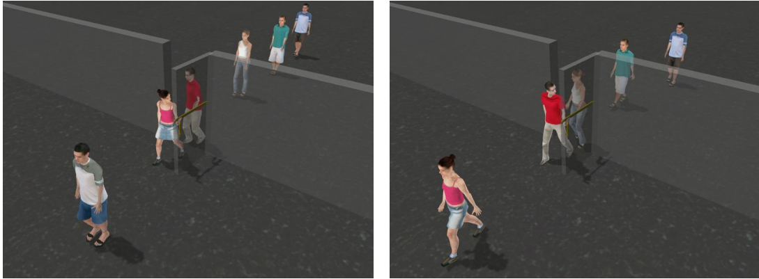
Figure 7.3: Sprung hinged door simulation (pushing side). (a) Continuous passing sequence generated by generally kind and unhurried pedestrians. (b) Frequently interrupted passing sequence by less kind but hurried pedestrians.
