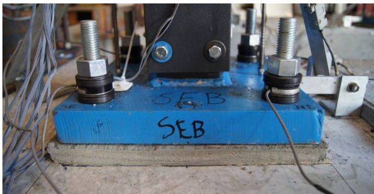
Figure 5-63: Configuration 2 - typical condition of baseplate connection in following all strong-motion tests
