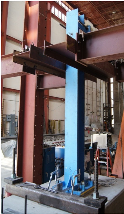
(a) Isometric view of column stub, and details of column base with variable stretch length
