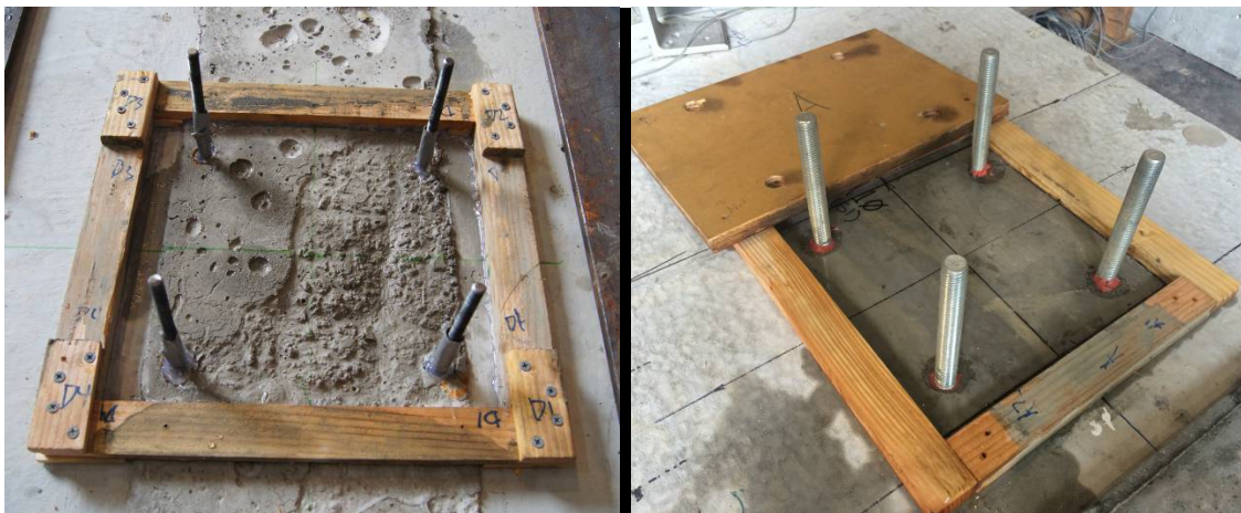
Figure 5-16: Grout forms for cast-in anchor stations with cutout (left) and post-installed anchor stations showing unfastened top plate (right)
