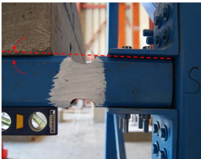
Figure 5-66: Configuration 2 - visible rotation of 1st-floor fuse in SW corner following Maximum motion
