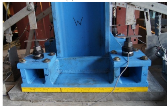
(c) Chair assembly providing 8 diameters (8D) stretch length
