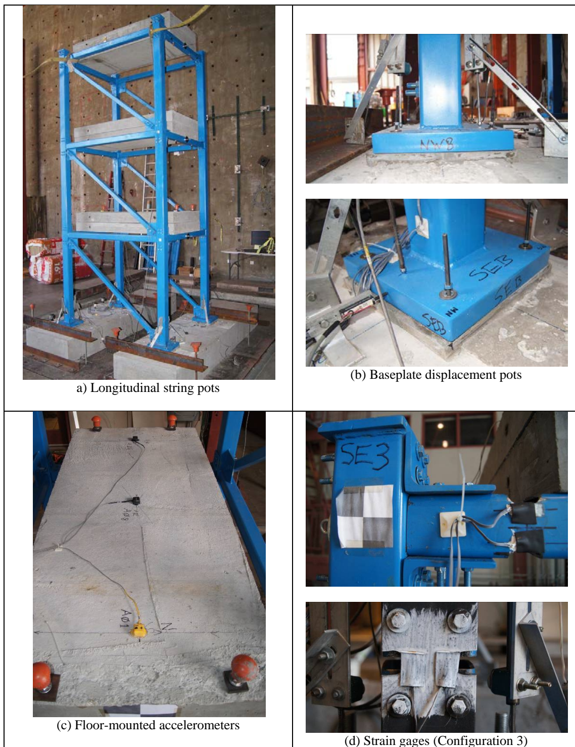
Figure 5-25: Photographs of instrumentation on specimen
