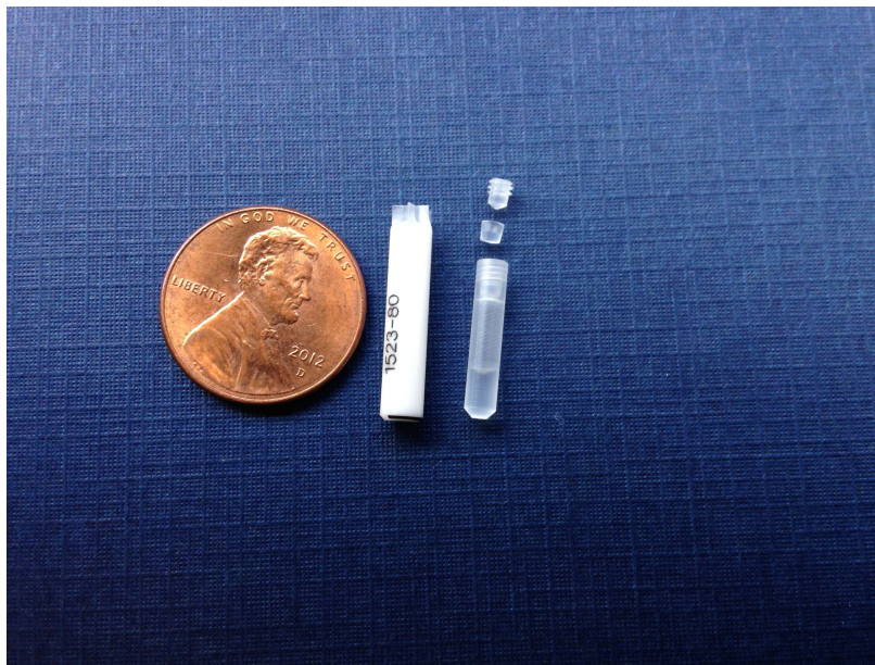
Figure 6.2: NMR rotor and rotor inserts used for samples containing depleted ^{238}\text{U} .
