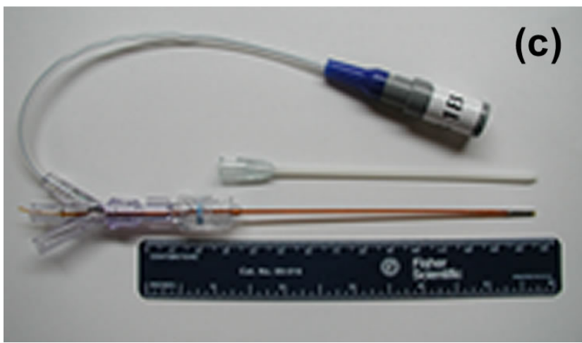
Figure 3.1: (a) Schematic drawing of a tri-sectored tubular ultrasound transducer with internal water-cooling. Pictures of (b) TriAD/DC and (c) TriAD/CC applicators constructed with polyimide tubing.
