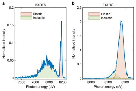
**Fig. 2 XRTS spectra.** The scattered X-ray signals are recorded with the (a) backward and (b) forward spectrometers, at scattering angles of 123° and 17° to the incident X-rays, respectively. The integrated areas for Eqs. (2) and (3) are shaded in red and green, respectively. Both spectra have been corrected for energy-dependent influences and are normalized to the integrated inelastic scattering measured on the backward spectrometer.
