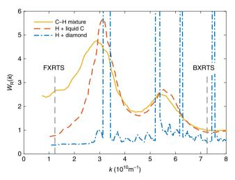
**Fig. 3 DFT-MD simulations.** Structure calculations for p=156 GPa and T=5000 K show a significant drop in the Rayleigh scattering  $W_{\rm R}$  for CH in a demixed state for  $k\lesssim 2.5\times 10^{10}$  m $^{-1}$  when assuming either liquid carbon or diamond in the pure carbon phase. The dashed vertical lines mark the wavenumbers probed by the spectrometers.
