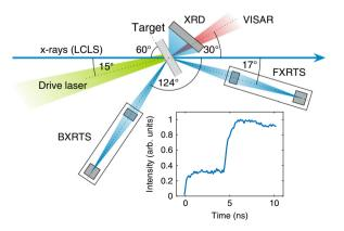
**Fig. 1 Schematic of the experimental setup.** The drive laser compresses the sample using a stepped pulse profile (see inset). The C-H separation is recorded in situ using XRTS and XRD simultaneously. The shock dynamics are constrained by an optical Velocity Interferometer System for Any Reflector (VISAR).
