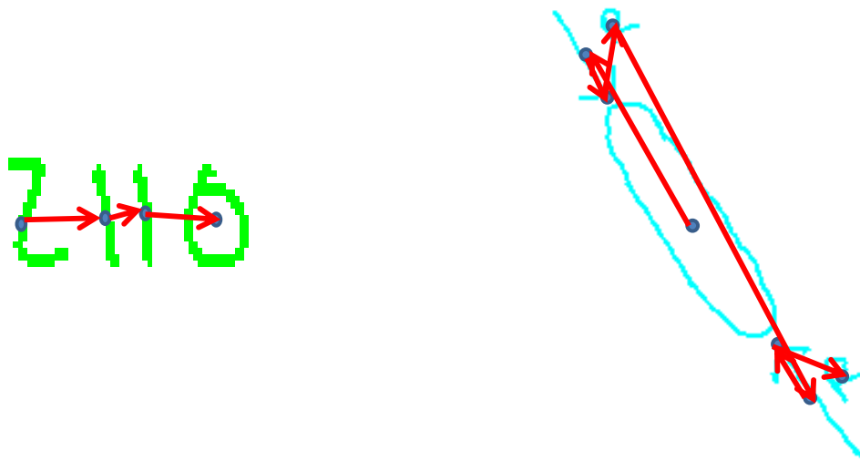
Figure 3.18: (Left) Red arrows show direction from the centroid of one pen stroke to the next in an equation. (Right) Red arrows show direction from the centroid of one pen stroke to the next in a free body diagram.
