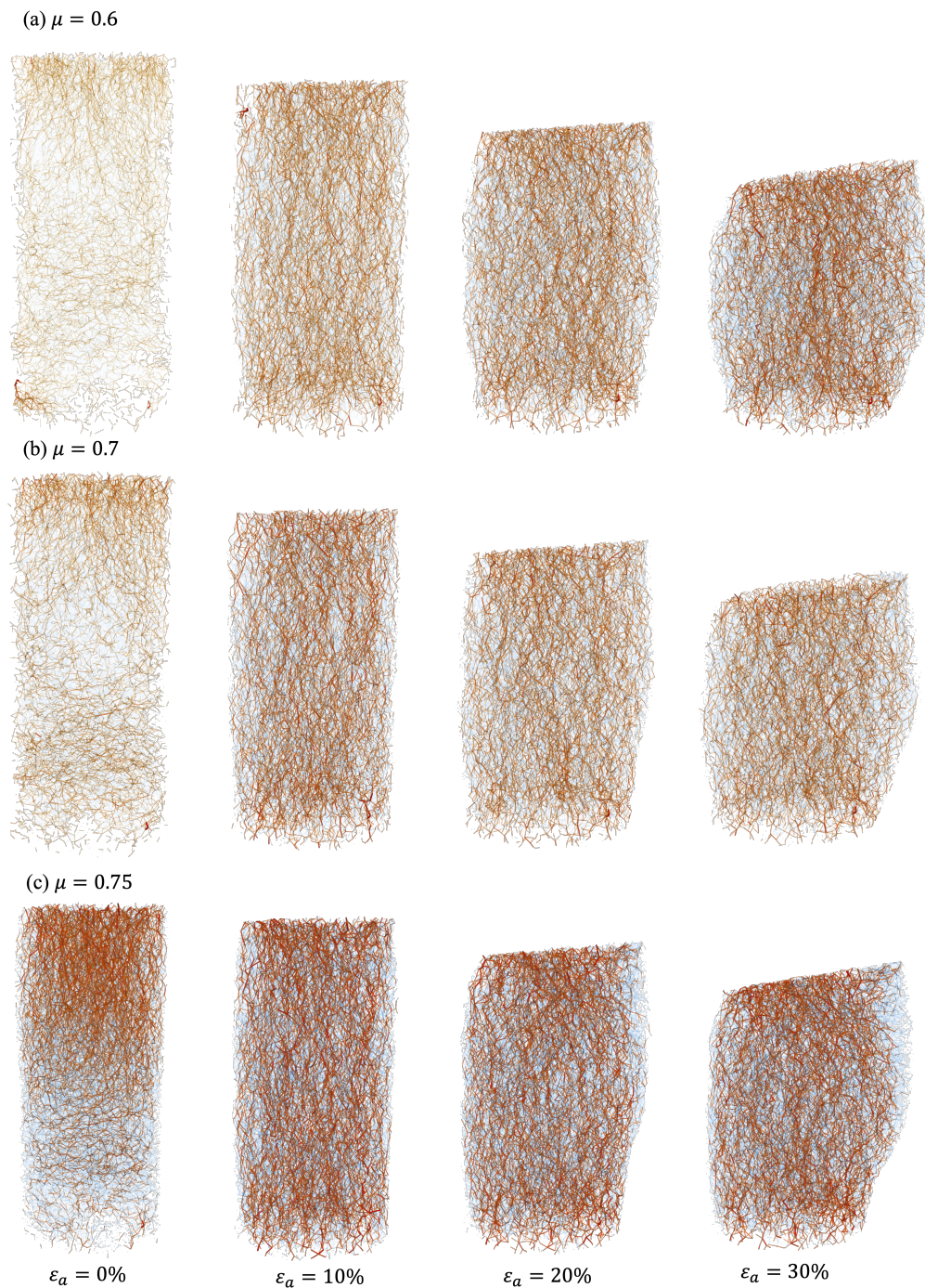
Figure 4.18: Force chain evolution obtained from low-resolution specimen between 0 ~ 30% axial shortening with internal friction coefficient, (a) \mu = 0.6 ; (b) \mu = 0.7 ; (c) \mu = 0.75 , forces change directions when they passing through the shear band.
