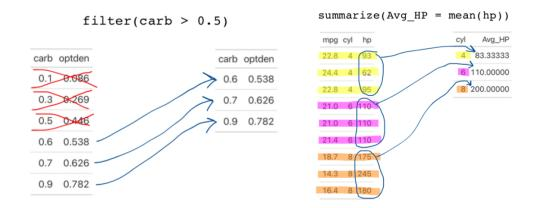
**Figure 6.1.** Hand drawn annotations showing how each function, with corresponding arguments, transforms a data frame from one state to the next. These kinds of illustrations inspired the illustrations created by Tidy Data Tutor.
