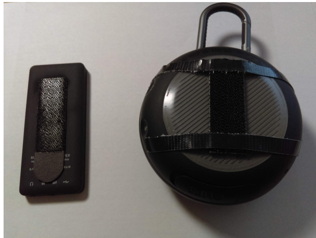
Use Velcro + tape to hold speaker and player together
