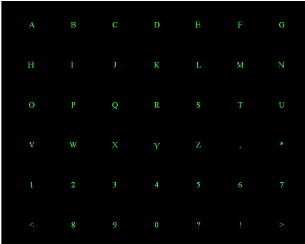
Figure 4.1: Layout of the P300-speller grid. Adapted from [1].
