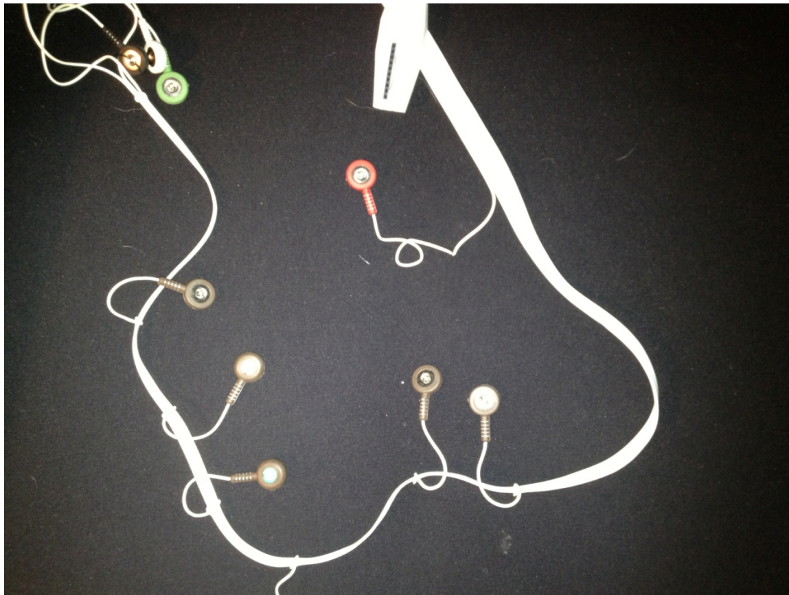
Figure-4.2—Patients preferred this type of single trunk electrode lead wires with branches that "peel" off (Mortara Instruments, Inc.)
