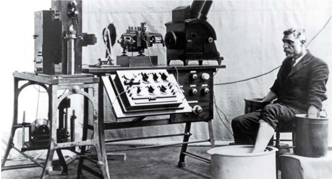
Figure 2.1 Einthoven string galvanometer for ECG circa 1912. Source: Hulton Archives, Getty Images, Downloaded from Wikipedia, Nov. 2013
