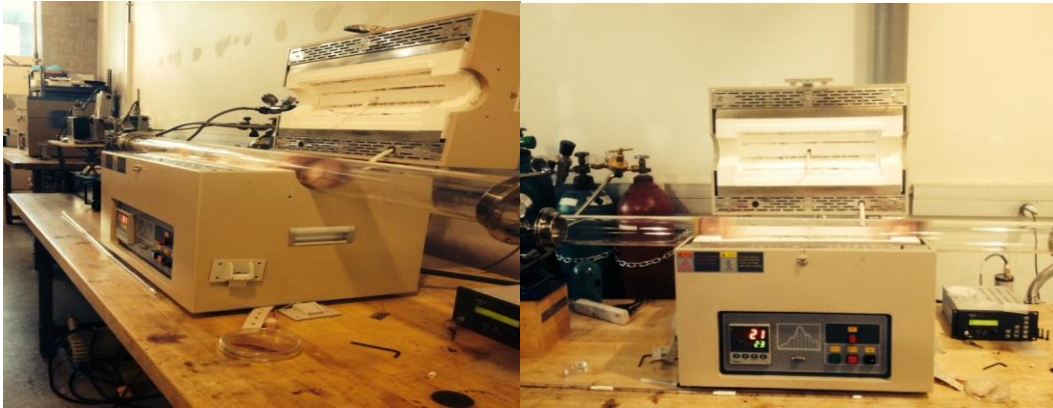
Fig 20: Original images of chemical vapor deposition furnace
