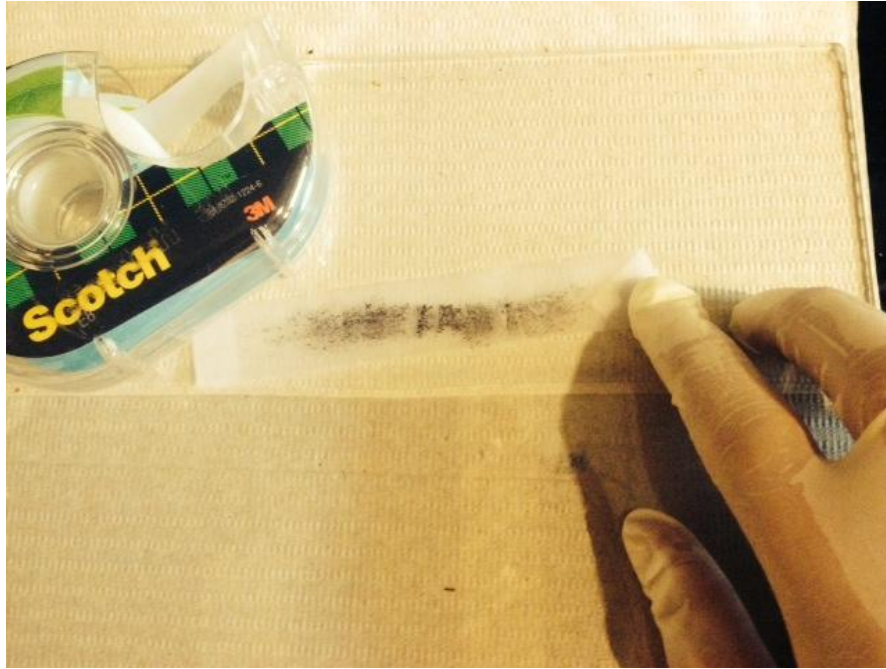
Fig 13: Exfoliated graphene technique. “Scotch” tape is pressed to the HOPG and folded several times.
