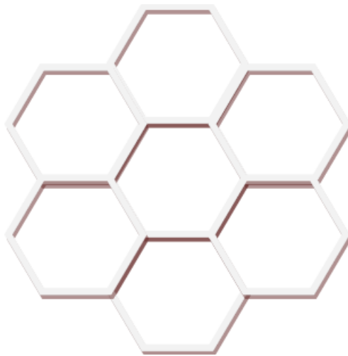
Fig1: Schematic of graphene
