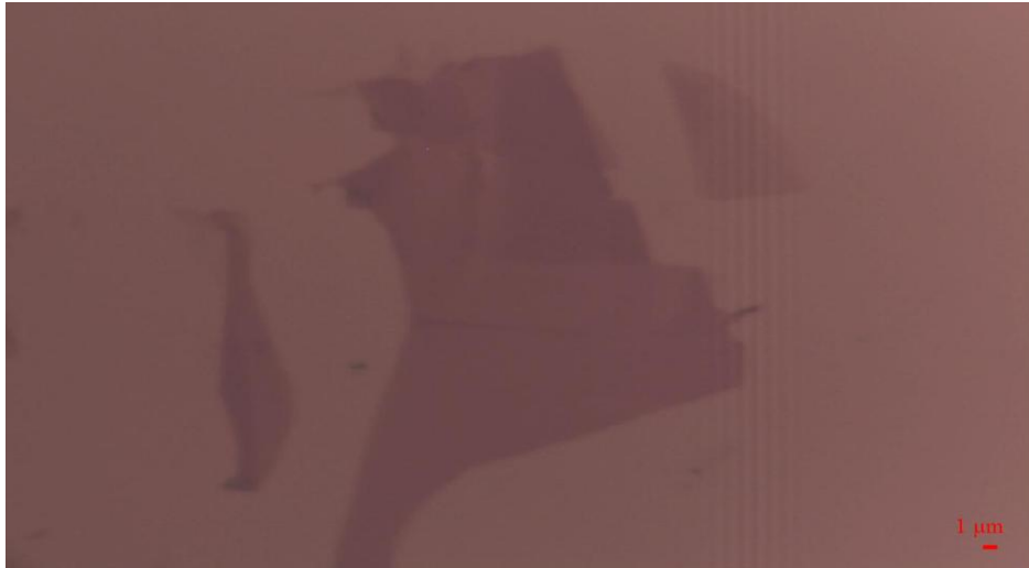
Fig2: Graphene standard optical microscopy image (100 x resolutions)
