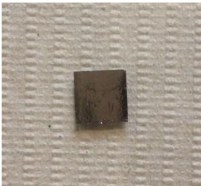
Fig3: HOPG wafer for making graphene flakes
