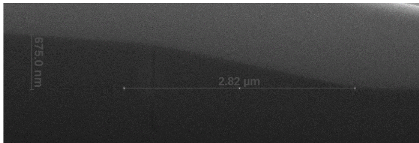
Figure 3.25: 45° angle (top) and 15° angle (bottom) etch profiles with thermal photo-resist reflow technique.
