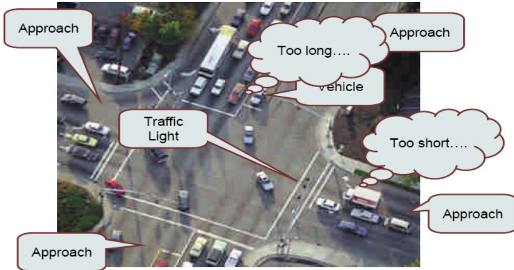
Figure 1.3: Safety related services in VANET: intersection collision warning
