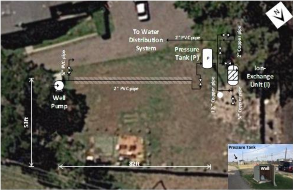
Figure E-1A: Schematic illustration of the existing water system layout in Blue Rock View Apartments (Note: community sanitary wastewater is discharged to a 4,500 gallons septic tank located 112 ft Southeast of the pressure tank.).
