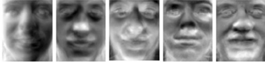
Figure 2.3: A representation of 5 individual eigenfaces, each representing the most influential features of a human face.
