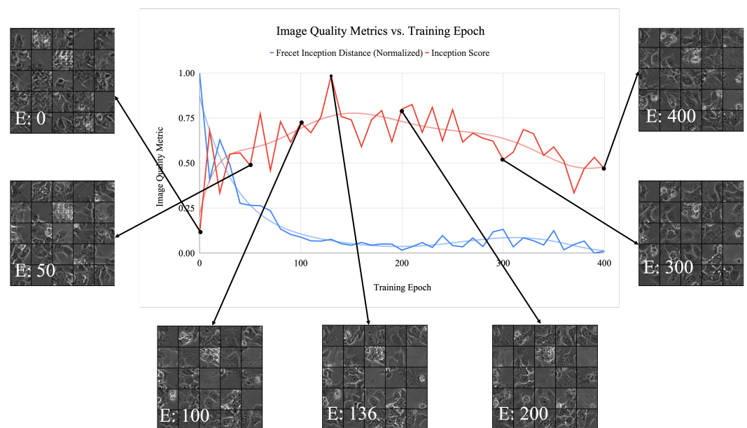
Figure 7. Normalized generator inception score (red) and FID (blue) per training epoch with example images at various intervals for the spread class. Graphs include accompanying trend line. Training epoch numbers are marked by a white 'E' in the bottom of each image. Agreement between inception score and FID can be seen in terms of their relative minimum and maximum values versus training epoch.
