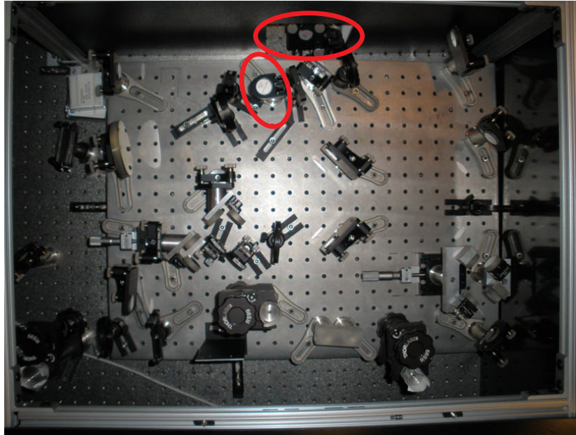
Figure 4.8: To observe the output of the interferometer with no shearing interaction, flip up these two mirrors.
