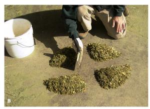
**Figure 4**. Dumping (A) and quartering (B) sample. The intermediate stage of mixing is not shown.
