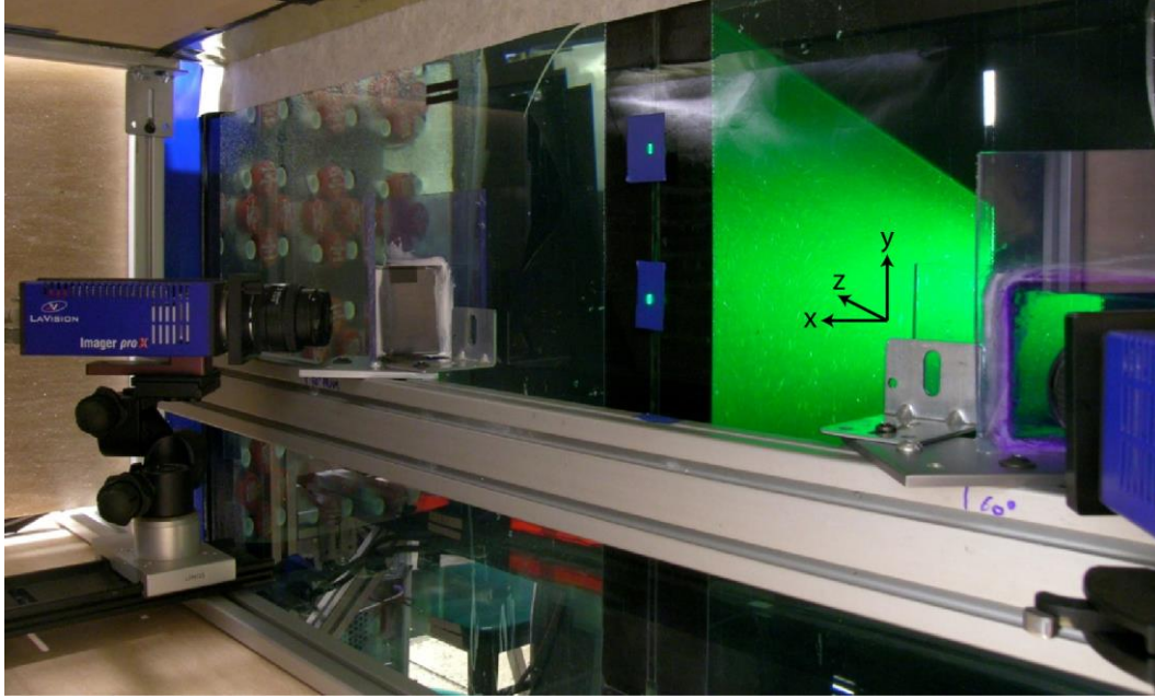
Figure 2.6: Photograph of imaging setup, showing cameras, Scheimpflug adapters, water-filled prisms, jet array, and laser sheet. A right-handed coordinate system is used as shown. Photo courtesy of Gabriele Bellani.
