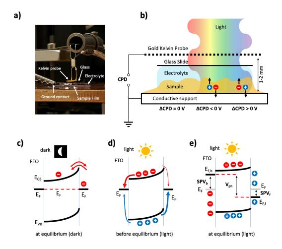
**Figure 2.** a) Vibrating Kelvin Probe Surface Photovoltage (VKP-SPV) Spectroscopy in liquids (Photo.) b) Schematic of the measurement configuration. Sample illumination occurs through the 60% semi-transparent KP, placed 1-2 mm above the sample, and through the electrolyte, enclosed by a microscopy glass cover slide. A water-saturated gas environment serves to prevent drying out of the electrolyte. The Contact Potential Difference (CPD) change under
