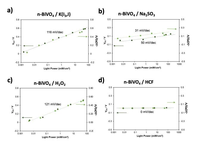
Figure 4. Open circuit potentials (Voc) and -ΔCPD values versus logarithmic irradiance (mW cm<sup>-2</sup>). Voc values were calculated from the data in Figure 3 and S5 using equation 4.
