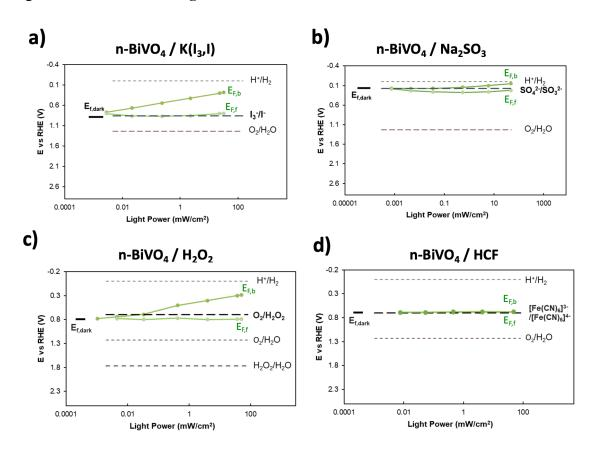
**Figure 5.** Plots of Fermi Levels  $E_{F,b}$  and  $E_{F,f}$  versus logarithm of irradiance.  $E_{F,b}$  values are from open circuit potential measurements in **Figure S5** and  $E_{F,f}$  values were calculated from SPV data using **equation 3**.
