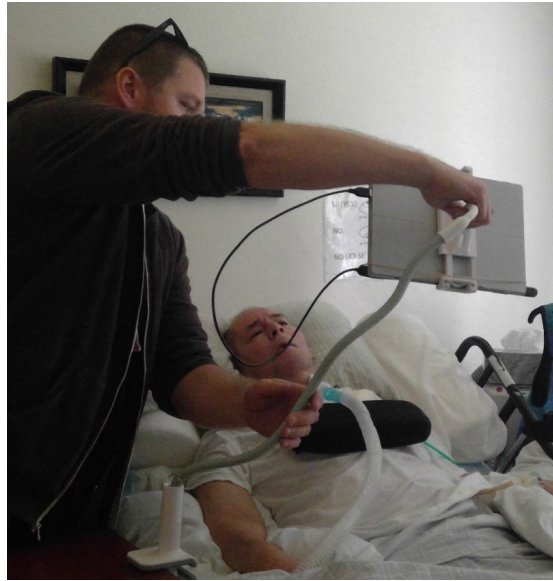
Figure 3.2: Setting up the Eyehome 3.0 data collection application on a tablet with an eye tracker, attached to a gooseneck clipped to a side table.
