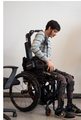
(c) The torso is light enough to be lifted like a backpack.
