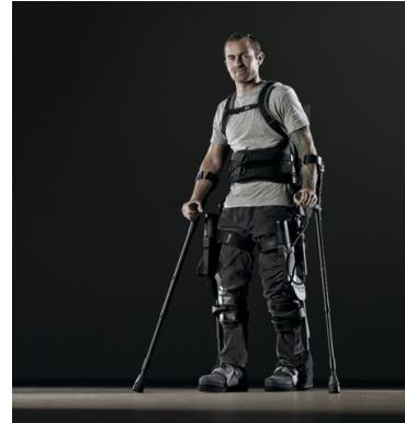
(b) Ekso (actuators: 4, weight: 45 lb, cost: $100,000)
