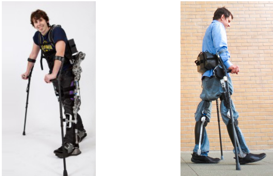
(a) The Austin exoskeleton used a mechanical coupling of the knee joint to the hip.
