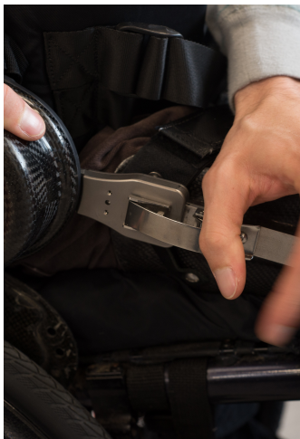
(d) The hip and leg braces are latched into place.
