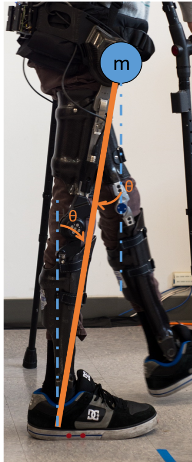
Figure 4.14: The simple model used for the stance leg.
