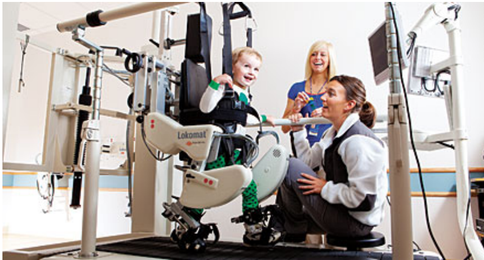
Figure 1.2: A child using the Lokomat, an in-clinic gait rehabilitation device [18].
