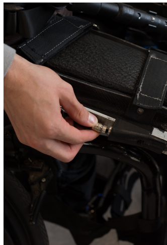
(e) The knee cable is connected to the knee.
