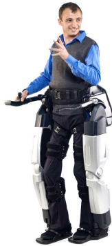
(a) Rex (actuators: 10, weight: 85 lb, cost: $150,000)
