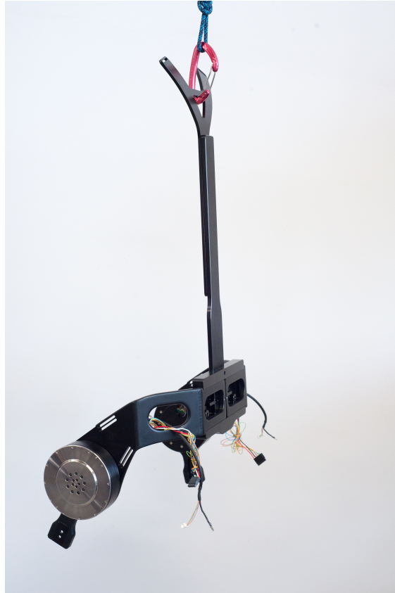
Figure 2.4: A stripped down version of the Phoenix torso piece showing the adjustability and minimal design.
