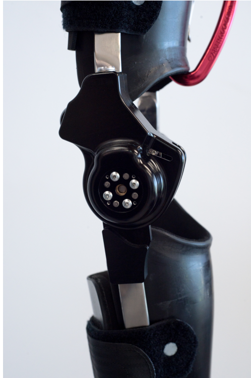
Figure 2.7: The Phoenix exoskeleton's lightweight, semi-passive knee mechanism.
