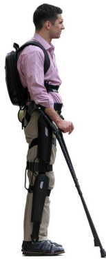
(c) ReWalk (actuators: 4, weight: 45 lb, cost: $70,000)
