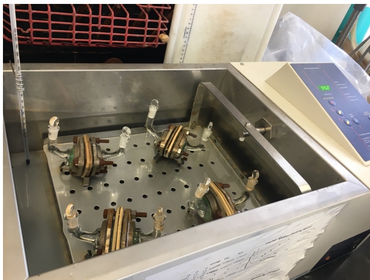
Figure 1. The Test Chambers in the Water Bath
