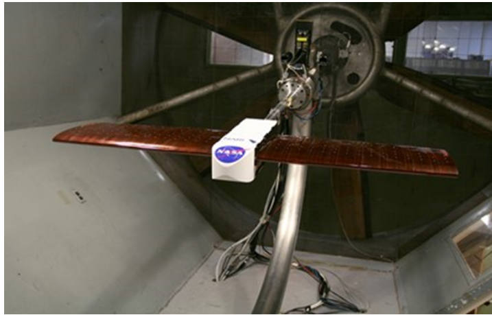
Figure 4.10: Active twist wing mounted in the wind tunnel
