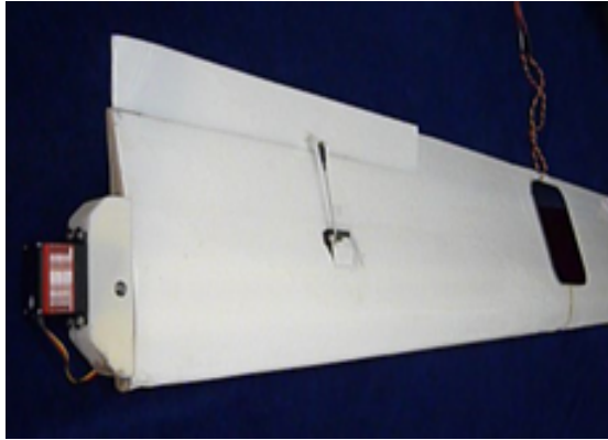
Figure 4.6: Twist capable and outfitted with an actuation system that enabled in-flight active twist demonstration
