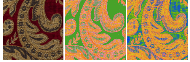
Figure 3: Initial and final sub-clusters for the two-camera red velvet lamé material. The left image shows the average color. Five clusters were obtained in the initial clustering (middle), and the final result included 5,152 sub-clusters (right).
