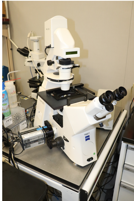
Figure 4.1: Fluorescence microscope used for particle tracking experiments.
