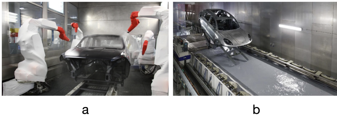
Figure 1.1: Examples of industrial use of external fields for painting and coating. a) Electrostatic spray painting of a car body, from [46]. b) Electrophoretic coating of a car body, from [47].
