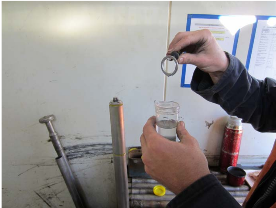
Figure 4.1.18. Stainless steel filter element being removed from silicone oil bath prior to installation.
