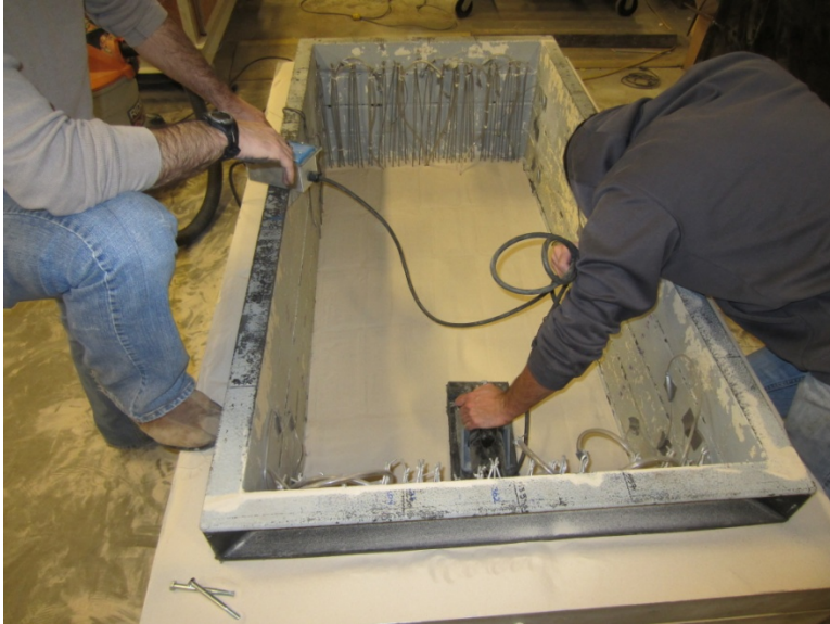
Figure 3.2.12. Vibration of dense Nevada Sand
