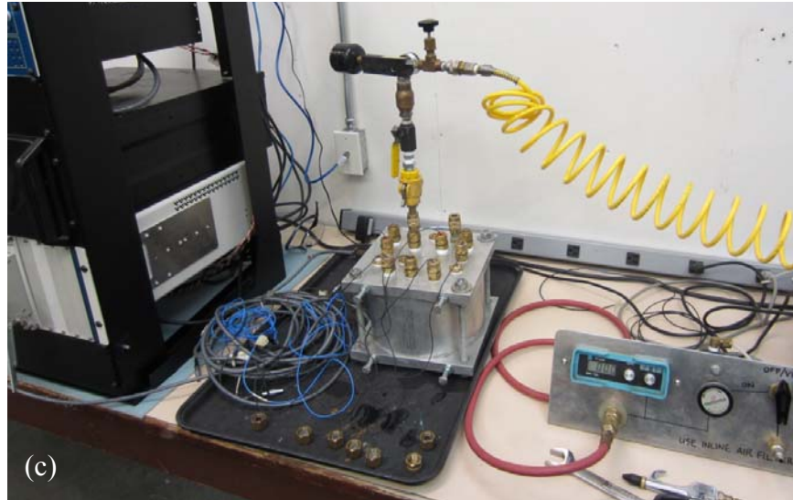
Figure 3.2.7. (a) Waterproofing ICP accelerometer with synthetic rubber. (b) View of the LP calibration station. (c) View of the PPT calibration station.
