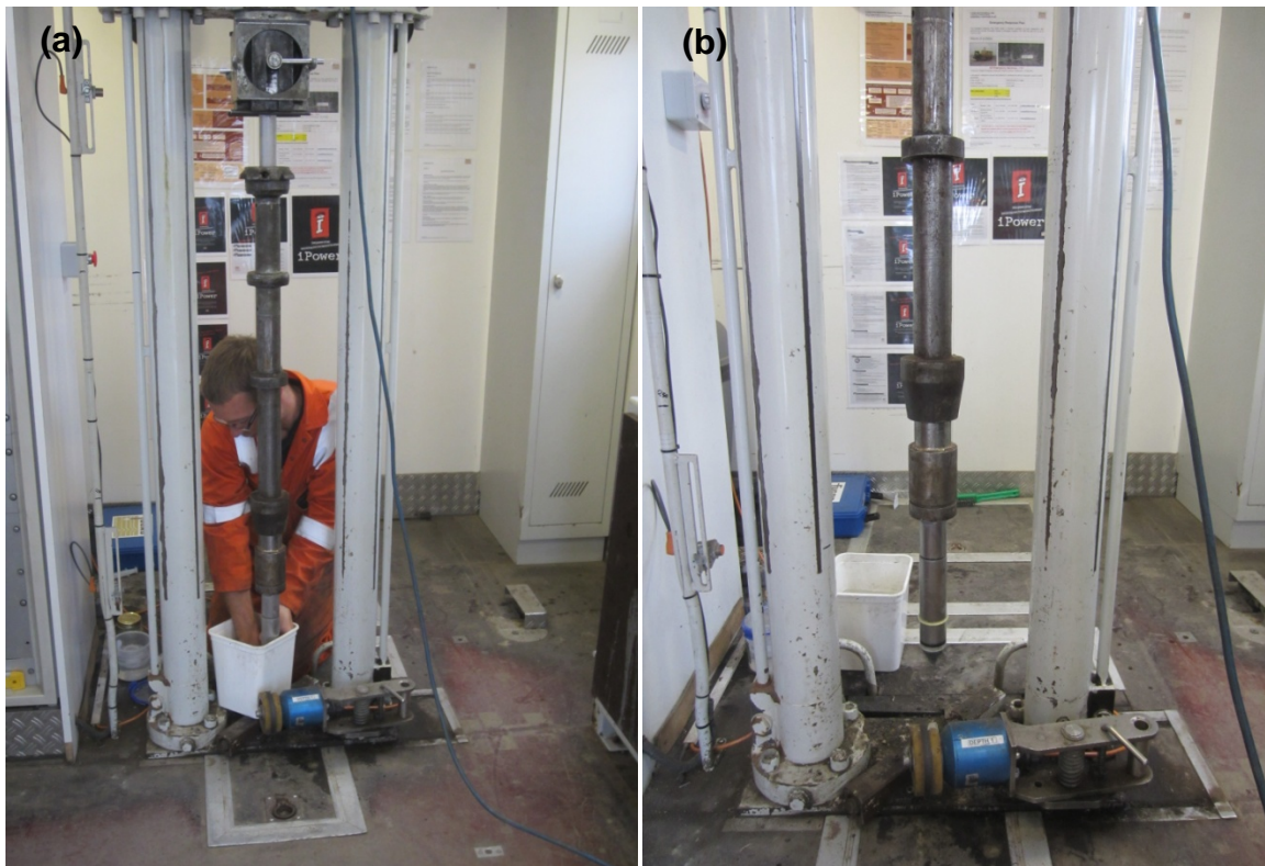
Figure 4.1.19. (a) Fugro filter element installation and (b) final assembly prior to CPTu.
