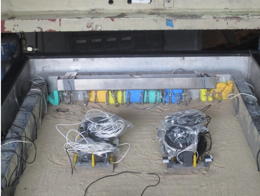
Figure 3.2.17. Sponges underneath saturation trough.
