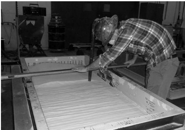
Figure 3.2.13. Vacuum soil lift to desired elevation.
