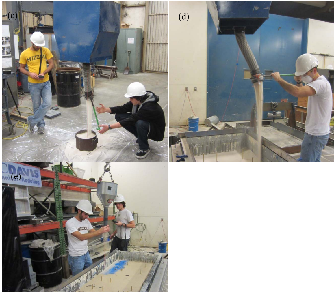
Figure 3.2.11. (a) Calibration of large pluviator. (b) Placing dense Nevada Sand using large pluviator. (c) Calibrating the pluviator for loose to medium-dense Nevada Sand. (d) Placing loose to medium-dense Nevada Sand. (e) Placing dense Monterey Sand.
