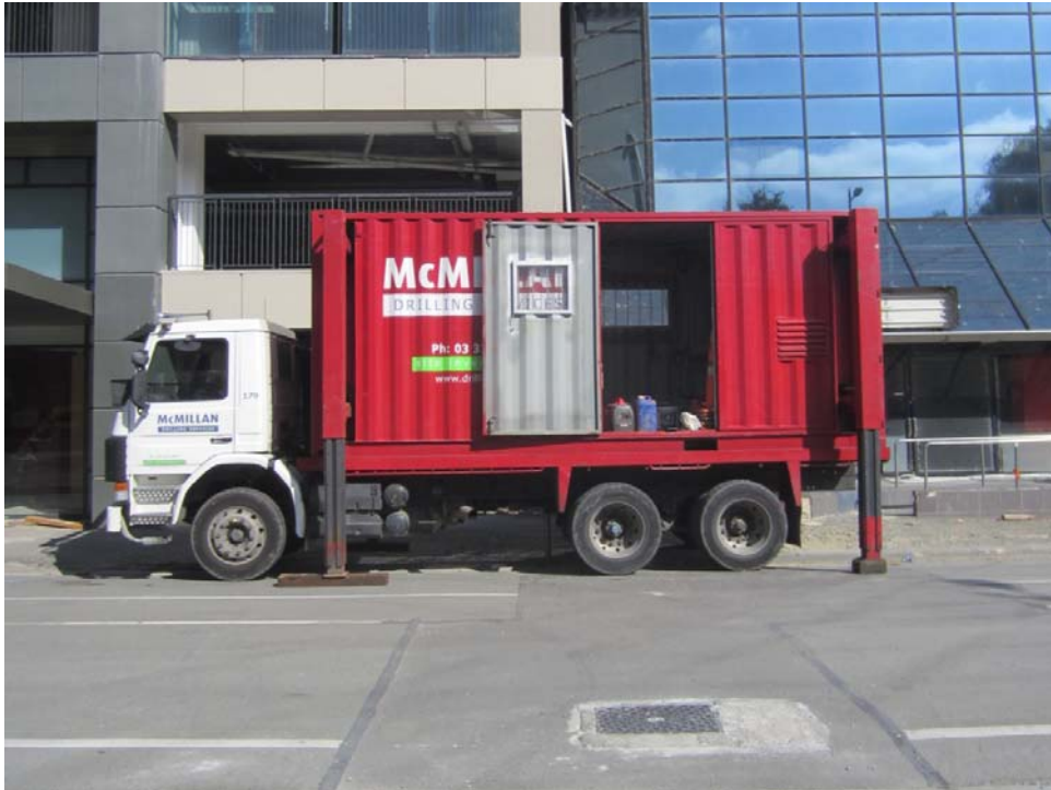
Figure 4.1.16. McMillan Drilling Services 22 Tonne CPT Truck
