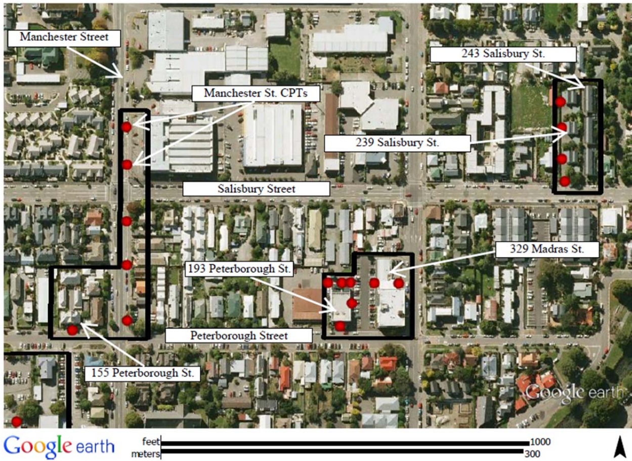
Figure 4.1.13. Zone 8 overview with structures of interest indicated. CPT locations are indicated in red.
