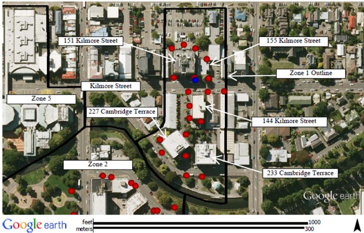
Figure 4.1.9. Zone 1 overview with structures of interest indicated. CPT locations are indicated in red. University of Canterbury borehole location indicated in blue.
