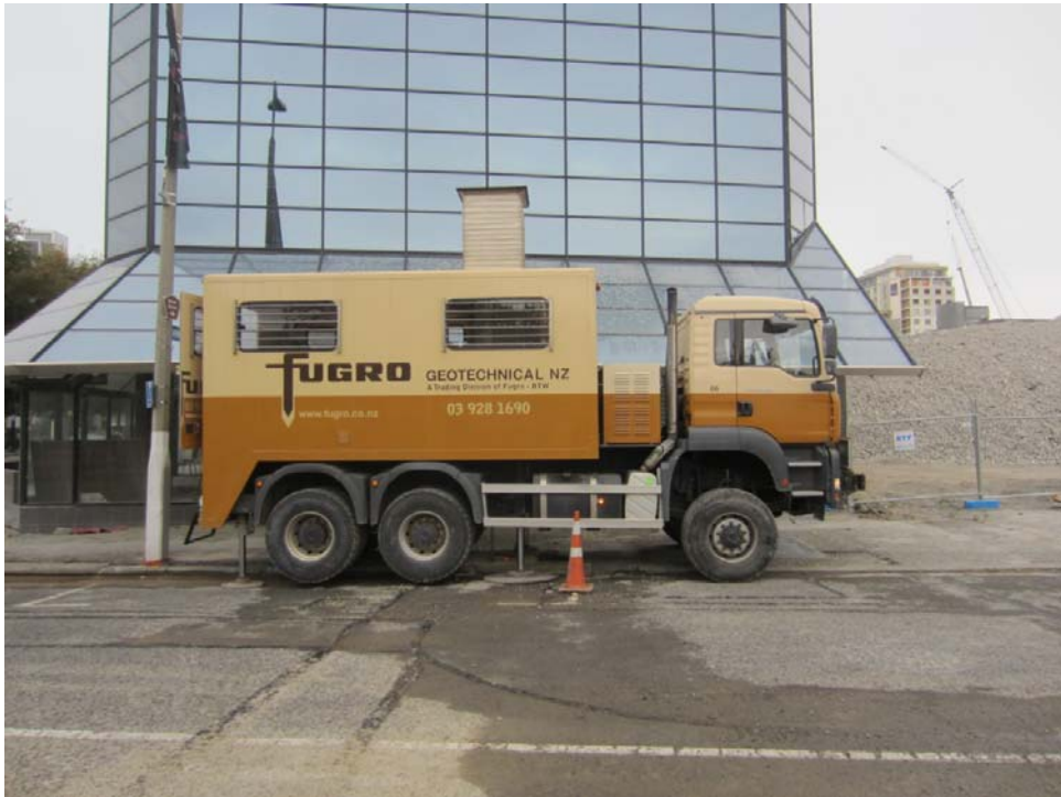
Figure 4.1.17. Fugro Geotechnical NZ 20 tonne CPT Truck.
