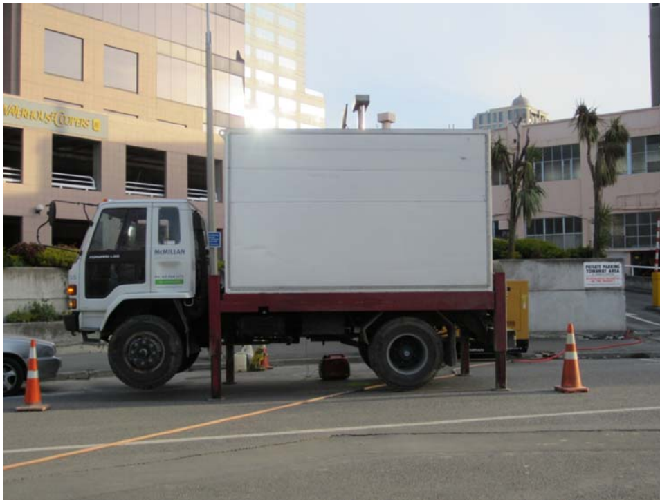
Figure 4.1.15. McMillan Drilling Services 14 Tonne CPT Truck
