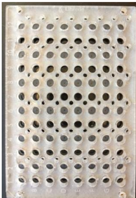
Figure 2-2 Top view of a multi-well bilayer array plate. The hydrophobic Delrin partitions can be seen in wells that will be loaded with organic solution; sessile droplets on pin tools are loaded into these wells; Aqueous wells contain a channel which flows directly underneath the organic solution wells; electrolyte solution is loaded into these wells through inlets located adjacent to the organic wells
