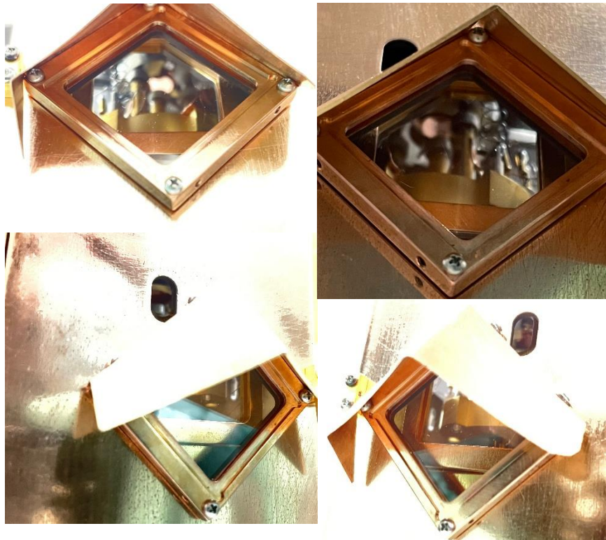
Figure A.15 Photos showing THz/optical path clearance and dosing hole clearance on both side of scanner with updated shield design
