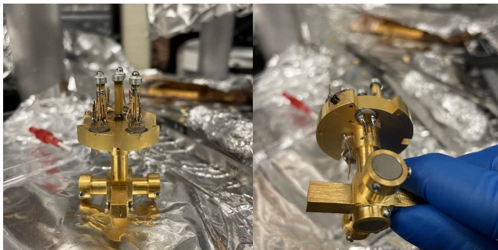
Figure B.3 Photos showing the new crosspiece mounted to scanner base plate.
