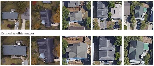
Figure 4.55: Comparison between original images from Google Maps and refined images produced by the roof segmentation model
