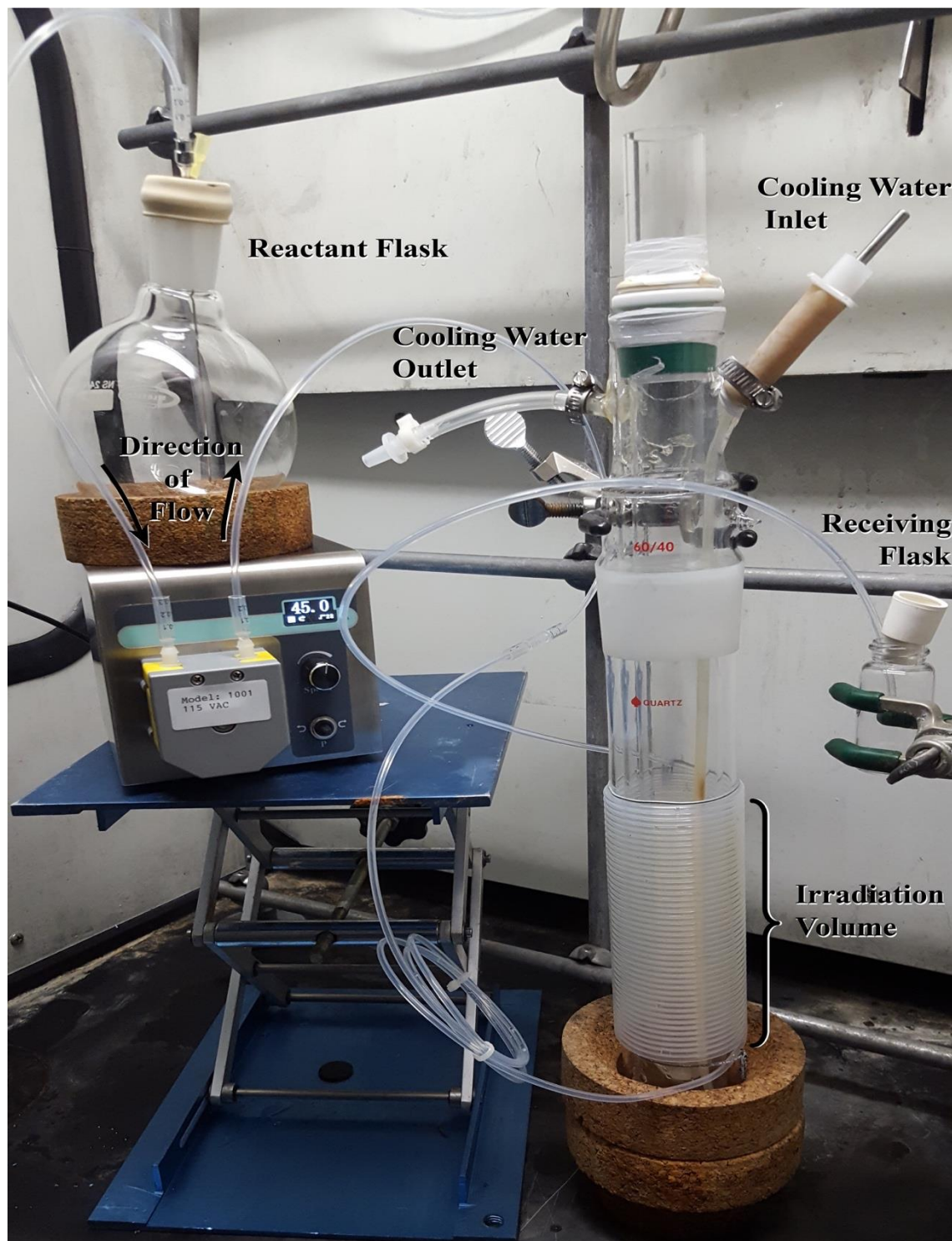
Figure 1.5.1. Setup of flow chemistry for photolysis.
