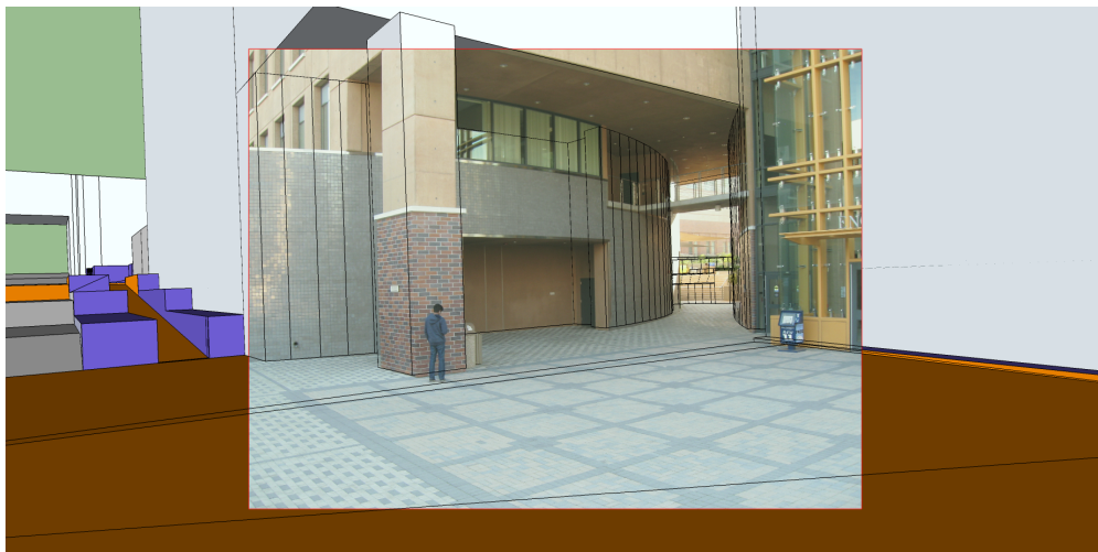
Figure 4.2: We developed a custom Sketchup plug-in that imports camera parameters computed during bundle adjustment. The user easily models the 3D geometry by extruding, tilting, and carving the 2D map data until it naturally aligns with the image.
