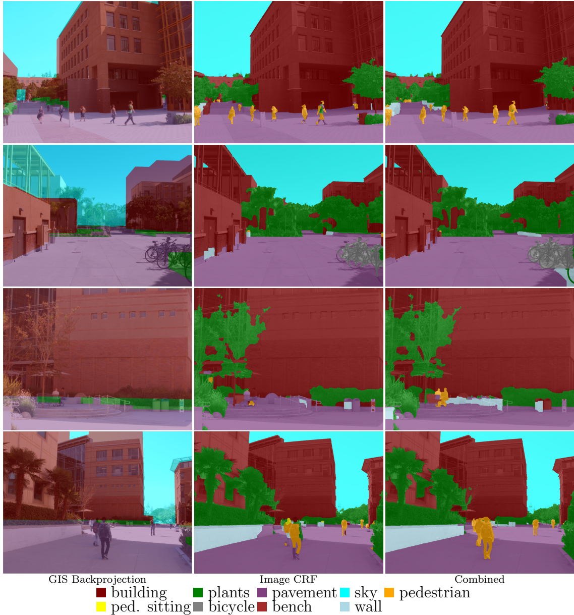
Figure 4.7: Qualitative segmentation results with overlaid images. Our combined model improves over a image-based CRF by incorporating features derived from GIS (depth, labels, normals) and a DPM detector.
