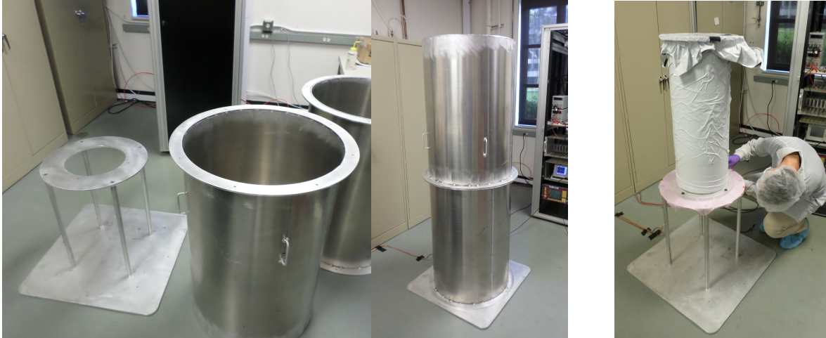
Figure 5.2: Left and Middle: The custom dark box built to house the Screener and detector stand. Right: The acrylic vessel as received being secured to the detector stand.
