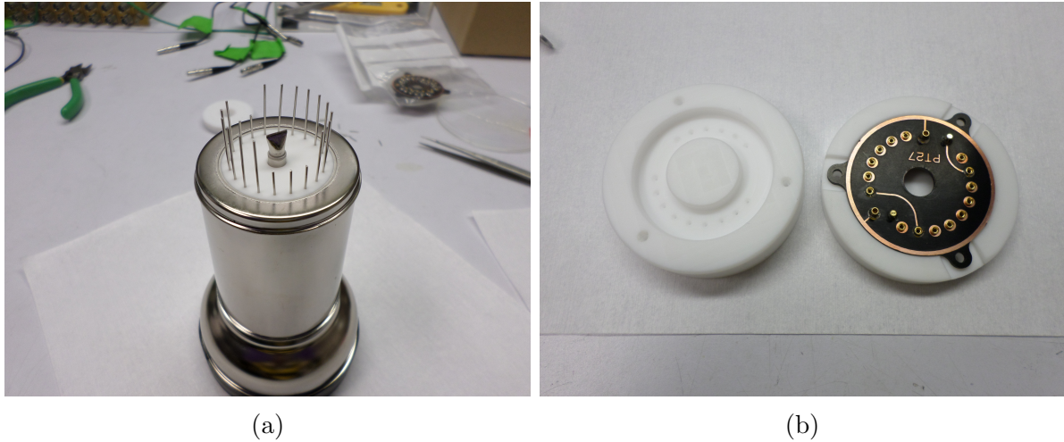
Figure 5.3: (a) A PMT with pins cut to length. (b) The PTFE pieces and a base.
