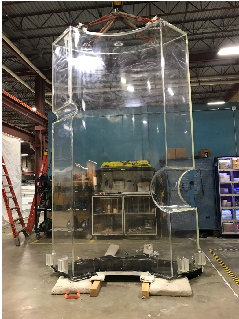
Figure 4.4: Photograph of an acrylic side tank for the LZ OD taken at RPT in Colorado. After the outside is cleaned, the tank will be wrapped with several protective layers for shipping and transport underground.
