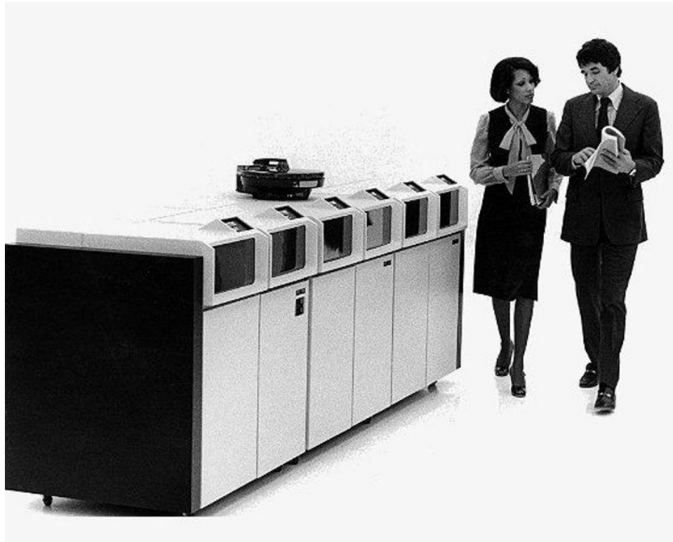
Figure 1.3 IBM 3340 Hard Disk Drive that used low-cost, low-load, landing read and write heads with lubricated disks [18]
