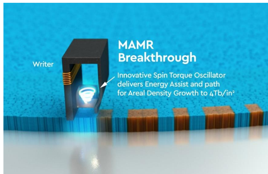
Figure 1.14 Schematic of microwave-assisted magnetic recording (MAMR). A spin torque oscillator (PSTO) is incorporated into the write element to deliver energy in form of AC field to the disk surface. Thus, the areal density of a MAMR drive can be increased up to 4\text{Tb/in}^2 [5]
