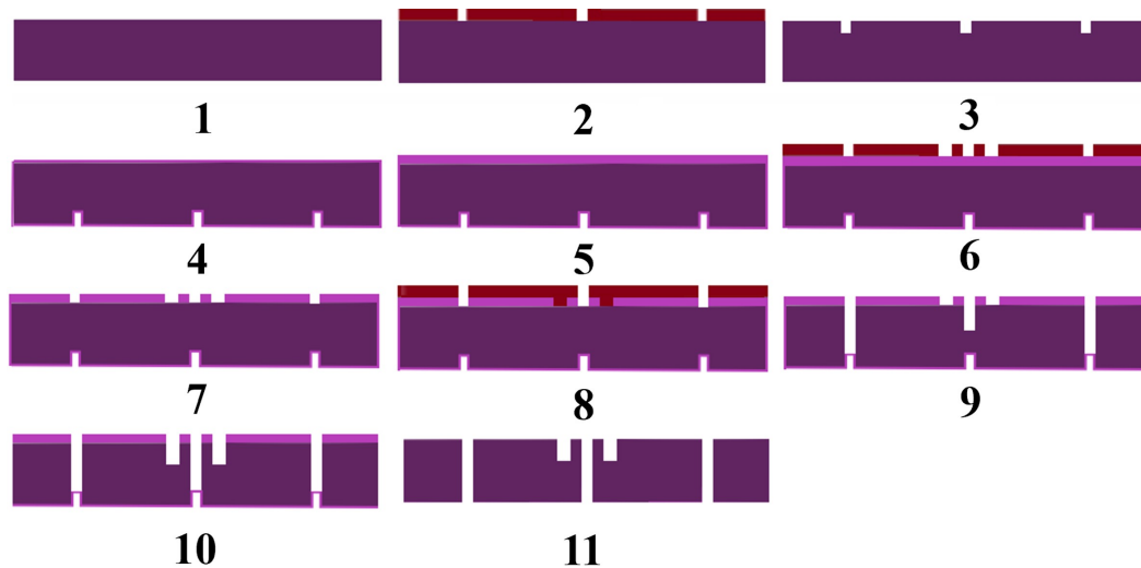
Figure 3.2: Schematic of the microfabrication process of the emitter array electrode.
