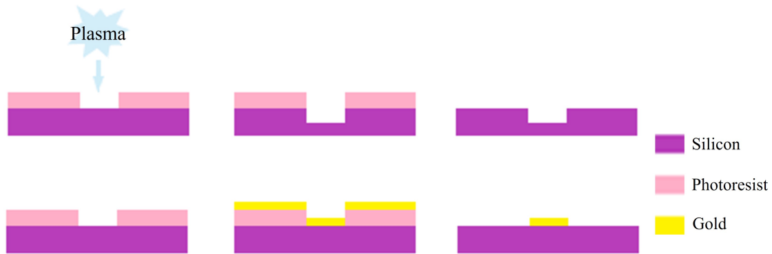
Figure 1.6: Schematic of a) DRIE and b) Lift-off process
