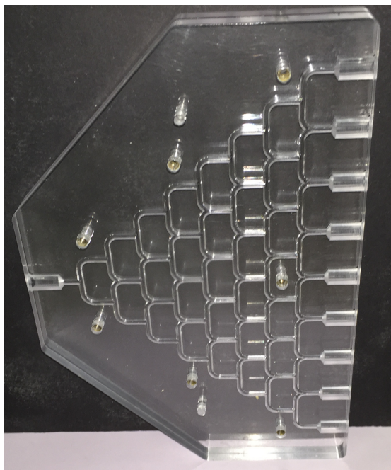
Figure 4.2: Second iteration of Hirsch-style maze, made of machined plexiglass
